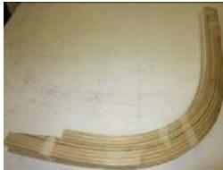
This is the first of two City and Guilds assessment pieces. You will loft the forward section of a small sailing dinghy, then take a template of the boat's stem from the lofting, using that template to set up a laminating jig to produce a laminated dinghy stem. The assessment includes a short written test.
